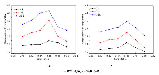
Figure 1. - Compressive strength of concrete at different ages with different sand ratios
