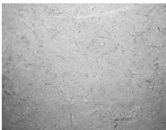
Fig. 2. Surface samples from the lime-silicate heat insulating fiber-reinforced concrete with a density of 800...900 kg/m 3
