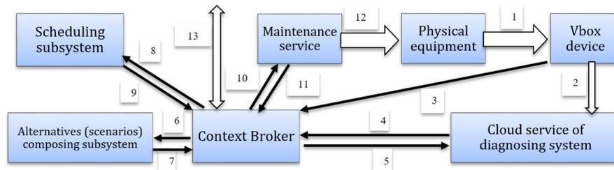
Figure 6. – Scheme of integration of vibration diagnosing system and business management system
