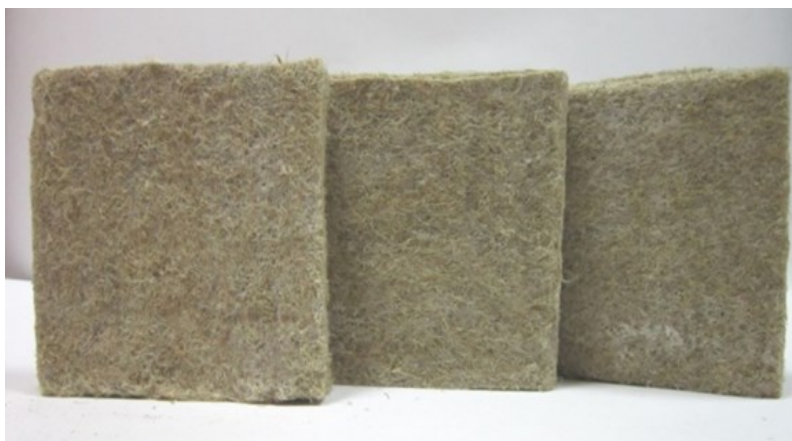
Figure 1. – Thermal insulation boards made of flax tow
