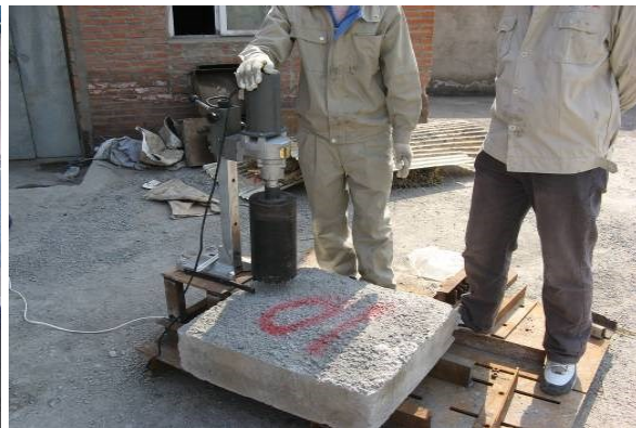
Figure 8. – Slab core drilling
