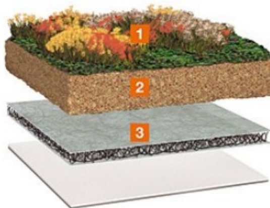
1 – landscaping; 2 – substrate - based on minerals 90% and 10% organic; 3 – protective, drainage and filter layer - Bauder SDF (polyamide drainage material - monofilament, drainage density 400 g/m 2 , material of the protective and filter layers polyester, density 200 g/m 2 , thickness 20 mm, total weight 600 g/m 2 )
